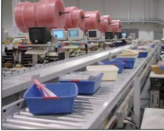
ing. "We had a takeaway line of conveyor that was loud, old and used," said Shopp. "It was minimum pressure accumulation, not zero pressure. It also had pass through gates people had to mess with to cross the conveyor line. We had tubs dump over on that conveyor. It just didn't accumulate right."
